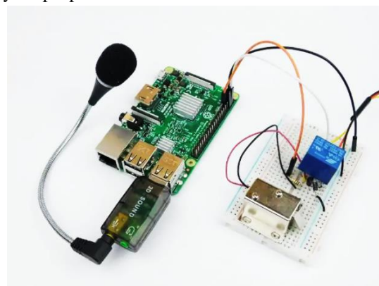
Fig 3: Voice Automation system connection
